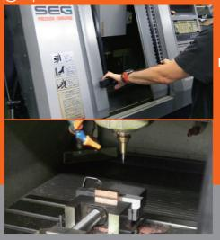
We perform cutting and electrical discharge machining to create the molds necessary for the
